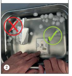
Pull the sensor out of the cover until the left light flashes once and insert it back into the sleeve
