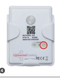
Activate thermometer and measure near the measuring point until the temperature remains stable
