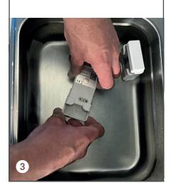
Alternative: Press and hold the activation button in the water for 2 seconds until the sensor flashes green once
