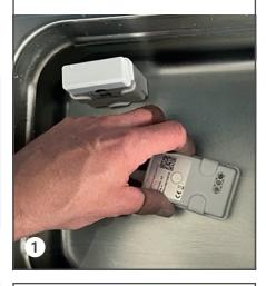
If necessary, weigh down the sensor to keep the measuring point under water
