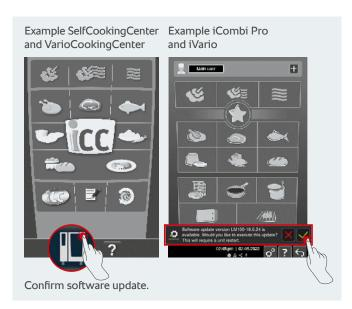
Step 2: Confirm automatic software update on the unit. New updates will automatically appear on the unit displays. All you have to do is confirm the update on the unit with just one tap, then it is carried out and the unit is restarted. The process is completed in a few minutes.
