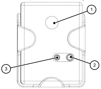
The WTS-12 also uses the light sensor to monitor the opening status of the fridge or warming cabinet and sends an alarm if the time is exceeded (five minutes by default).
